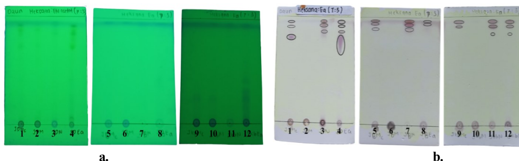
Figure 1. Chromatogram of the extract observed under UV light at 254 nm (a), after spraying with 2% CeSO 4 and heating (b)
