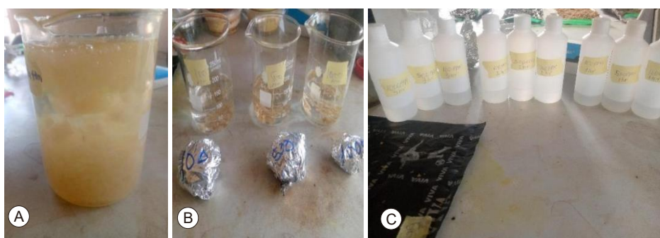
Figure 4. Formation of nanoparticle bits (A), Different concentrations of nanoparticle bits in waste water (B), and remediated water with different concentrations of nanoparticles and contact time (C).
