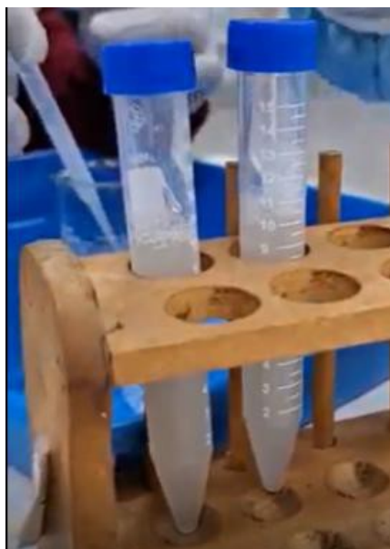
Figure 1. Process of lectin extraction from bean seeds using 0.9% physiological NaCl solution. Clear yellowish filtrate without sediment indicates successful separation of soluble protein fractions.
